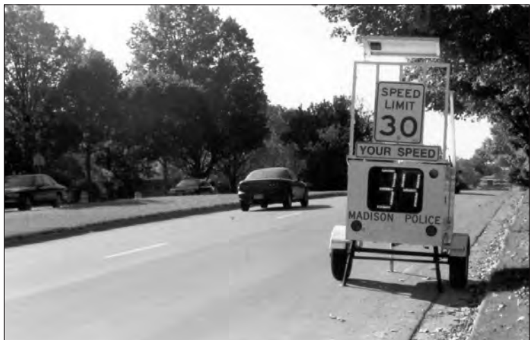
Speed display boards are a cost-effective way to reduce speeds.
