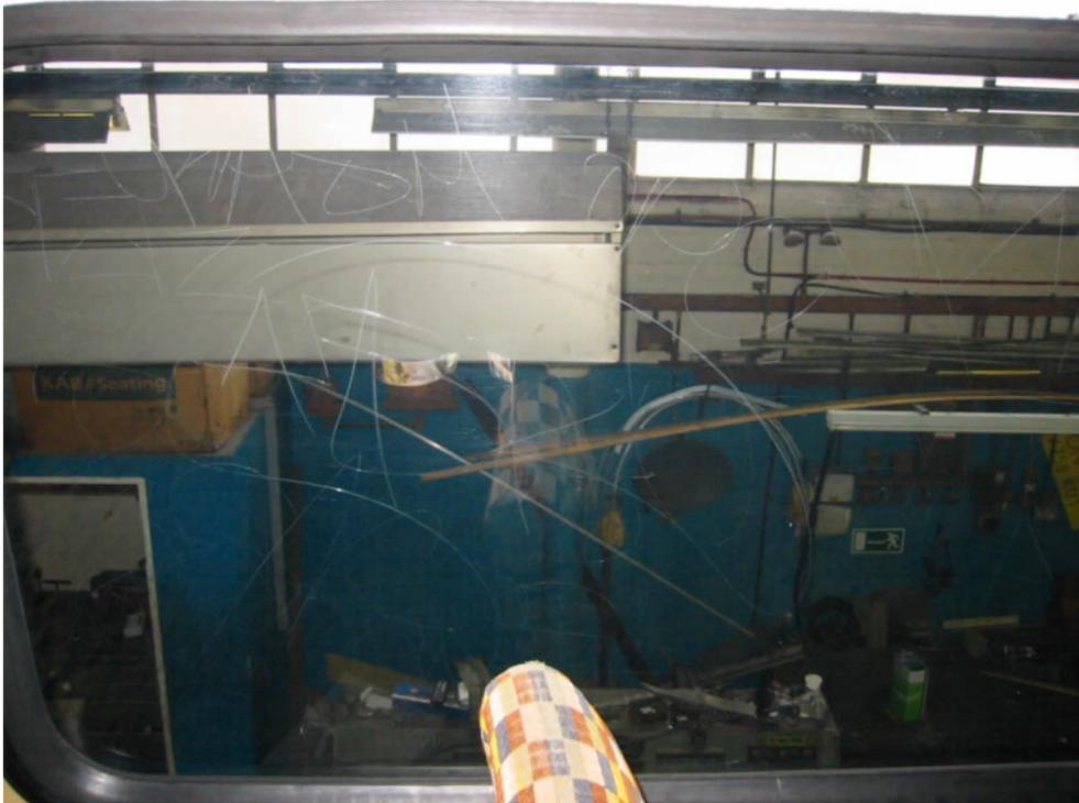
**Picture 1.** Example of Bus Vandalism – Scratched windows, replacement cost of up to £500 each.
