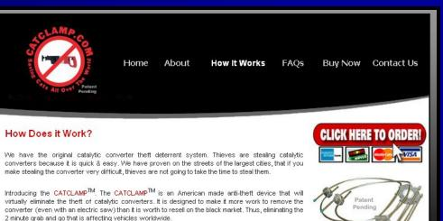
How does it work? The CATCLAMP<sup>TM</sup> essentially creates a cage around the catalytic converter. Two alloy collars lock at both ends of the converter. Special aircraft cable then runs between the collars making a cage around the converter. That same aircraft cable then locks the whole unit to the vehicle
