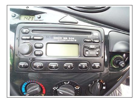
The above photograph shows the insertion of the four allen screws the top right only partially inserted ensuring the U clips no long fit into the holes. Also shows the unit has been marked with a post code.
